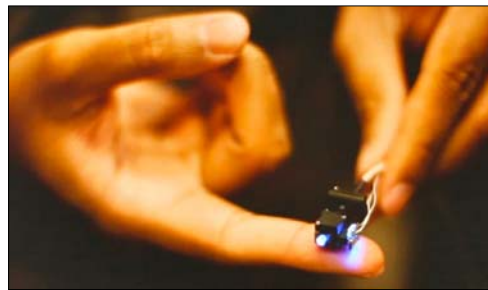
The image above shows the tiny microscope used in this study. The microscope is connected to a camera chip, which then sends a digital version of the image to a computer. (Image courtesy of Dr. Mark Schnitzer)
